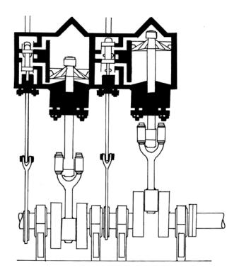
Reciprocating steam engine means equipment that is driven by steam acting on piston causing the piston to move, and includes an expanding (steam) reciprocating engine.
