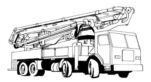
A concrete placing boom is plant incorporating an articulating boom, capable of power operated slewing and luffing to place concrete by way of pumping through a pipeline attached to, or forming part of, the boom of the plant.
