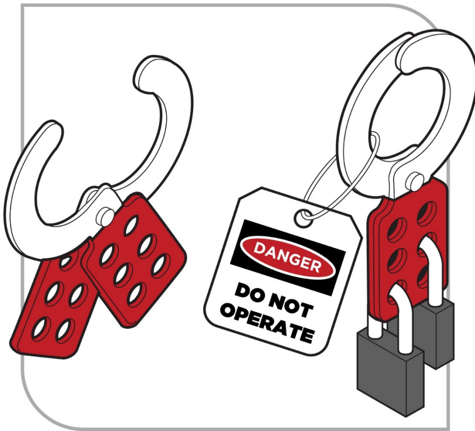
Figure 3 Example of tag and lockout with padlocks
