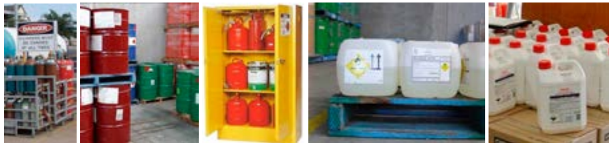
Gas cylinders, steel drums, and various bottles and small containers are examples of packages
