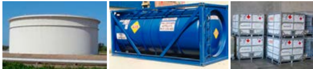
Static tanks and transportable containers such as isotainers and intermediate bulk containers (IBCs) are examples of hazardous chemicals containers requiring a bulk placard
