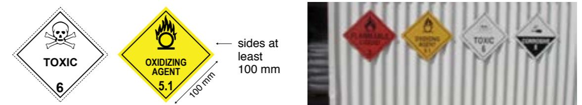
Figure 6. Example placards for a storage location for hazardous chemicals in packages
